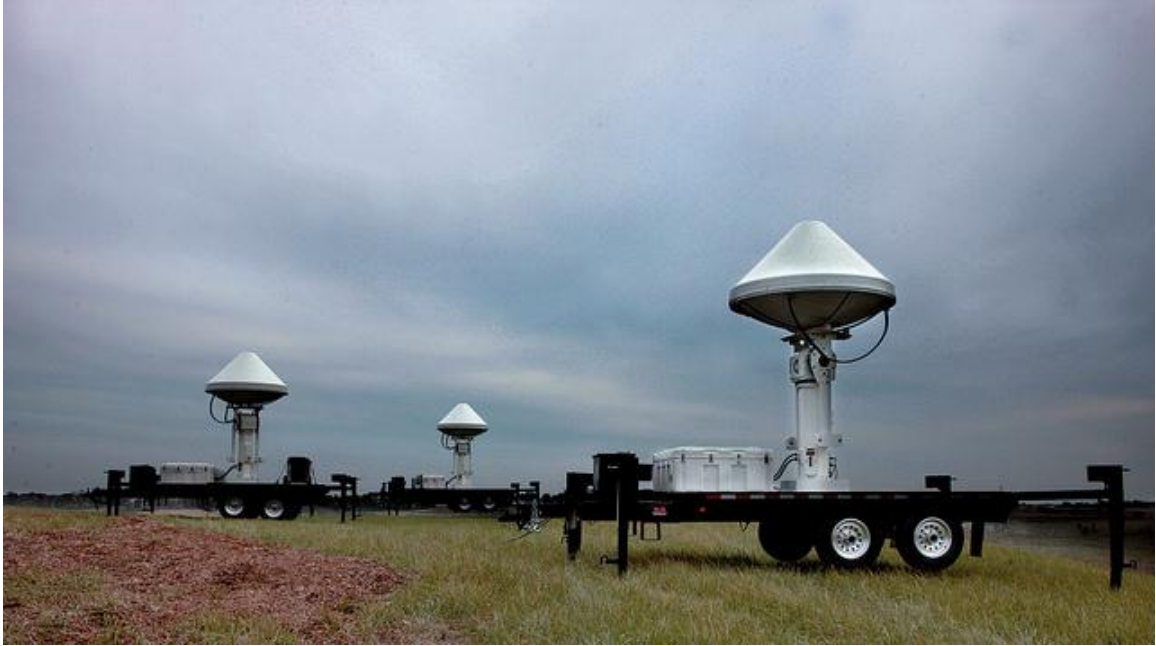
Figure 5.1: Radars of the University of Iowa Polarimetric Radar Network at the Iowa City landfill during the calibration experiment (April 2011).
