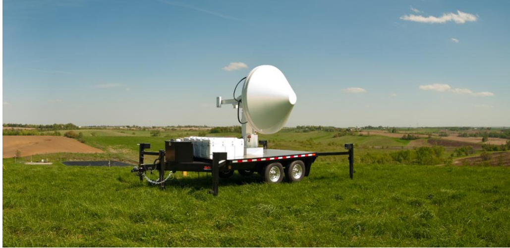
Figure 4.1: X-band polarimetric radar network node at Iowa City landfill.
